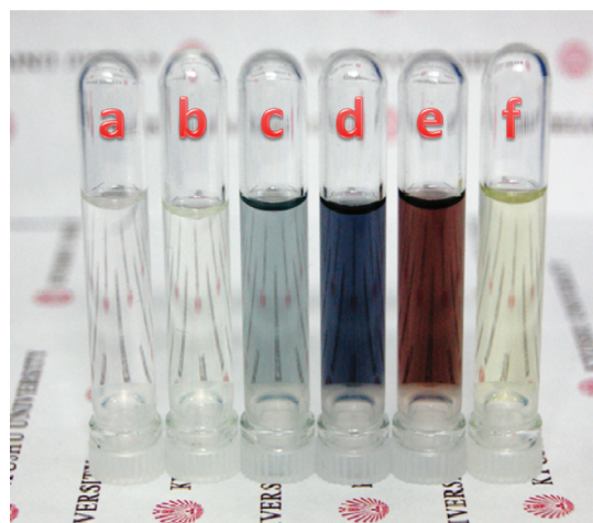
Figure 2. Photographs of 2 wt % copolymer THF solution with different amount of \text{Fe}^{3+} and MeONa, (a) 2 wt % copolymer THF solution, (b) [\text{Fe}^{3+}]/[\text{catechol}] = 0.33 , (c) [\text{Fe}^{3+}]/[\text{catechol}] = 0.33 , [\text{MeONa}]/[\text{catechol}] = 0.5 , (d) [\text{Fe}^{3+}]/[\text{catechol}] = 0.33 , [\text{MeONa}]/[\text{catechol}] = 1.5 , (e) [\text{Fe}^{3+}]/[\text{catechol}] = 0.33 , [\text{MeONa}]/[\text{catechol}] = 4.5 , and (f) [\text{Fe}^{3+}]/[\text{catechol}] = 0.33 , [\text{MeONa}]/[\text{catechol}] = 4.5 , with excessive acetic acid. UV-vis data for these samples at the lower concentrations are shown in Supporting Information, which gives the spectroscopic evidence for the reversible coordination in the copolymer system.
